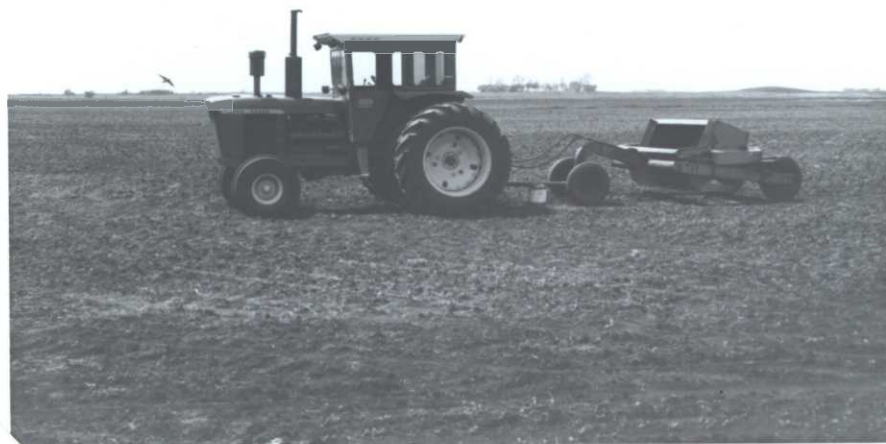
Small farm scrapers such as this have had a tremendous impact on wetland drainage. They are readily available and lower drainage costs considerably. JWH 10-68
