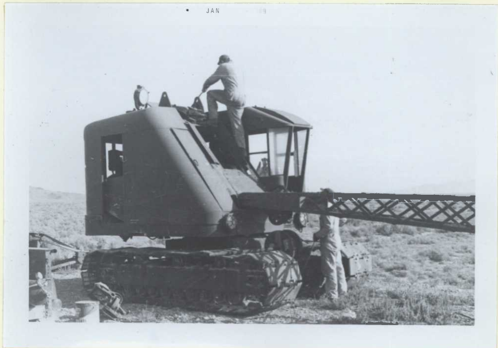
Refitting Byers Dragline with new cable and other assorted small parts. The wide tracks on this machine are a great help in our marshy areas.
