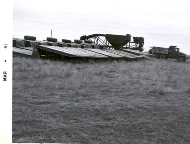
R. 8, Exp. 12, April, 1961. Five semi-trailers & a gravel bin obtained from Army surplus. The trailers are 10' wide & will be converted into bridges. The gravel bin will be cannibalized for the three excellent conveyors in it. Four similar trailers were obtained for the Fort Niobrara Refuge.
