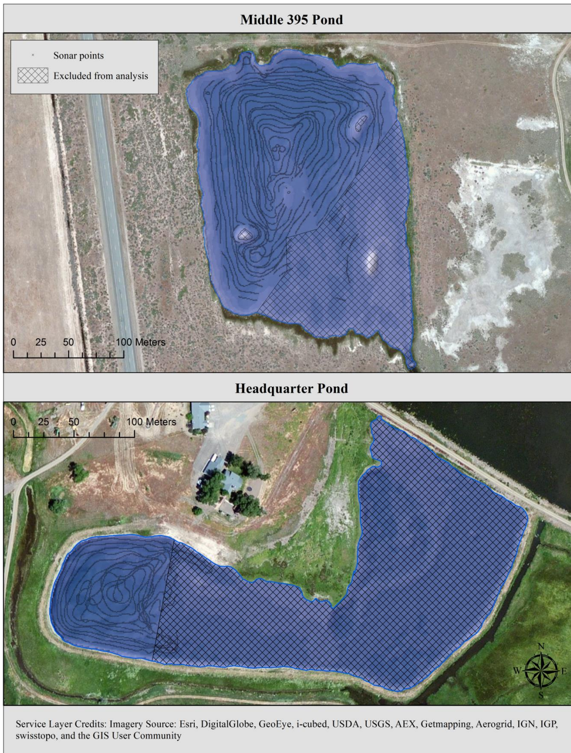
Figure 3. Map showing sonar survey coverage and area excluded from analysis in Middle 395 Pond (above ) and Headquarter Pond (below).
