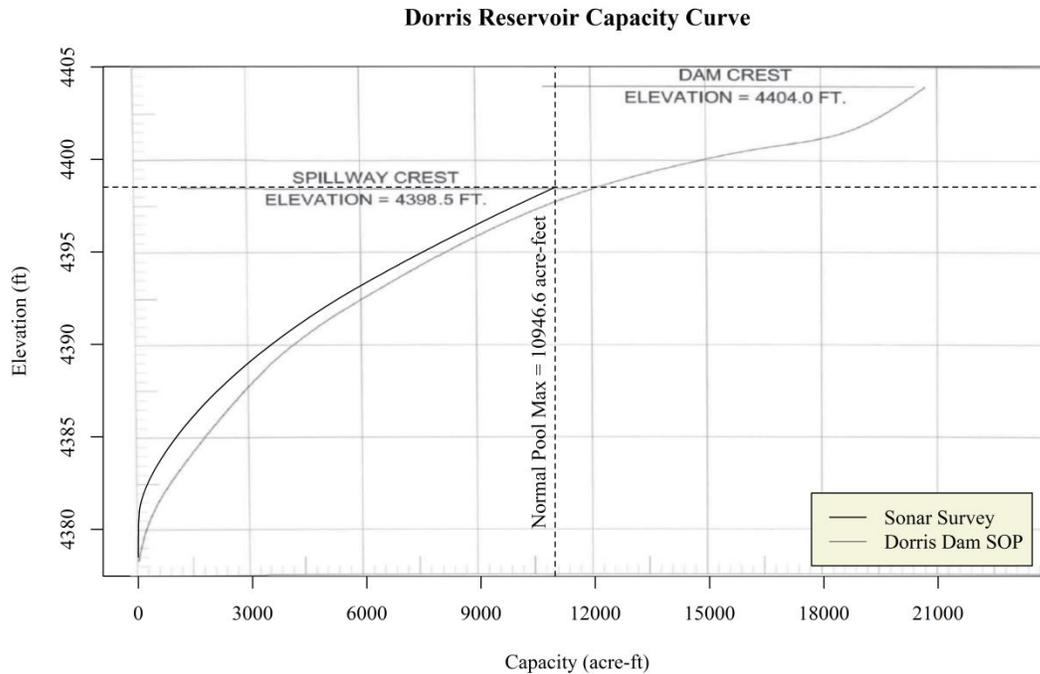
Figure 5. Reservoir storage curve from the sonar survey plotted over the existing storage curve from the Dorris SOP document for comparison. There is some minor distortion in the background image, but the general trends can be compared.
