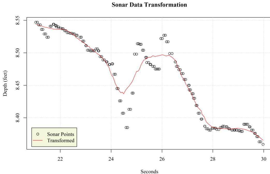
Figure 2. Sample of the raw sonar data transformation using a moving window average with a span of 1 second.
