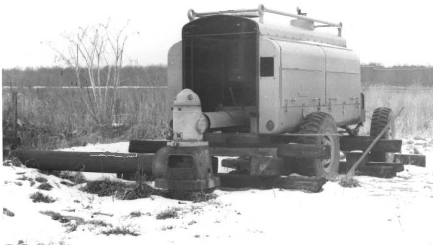
Figure 10. Audrey Walk, our heavy duty mechanic, converted a surplus air compressor and power unit into a water pump power unit at an estimated cost savings of $2,300.00.
