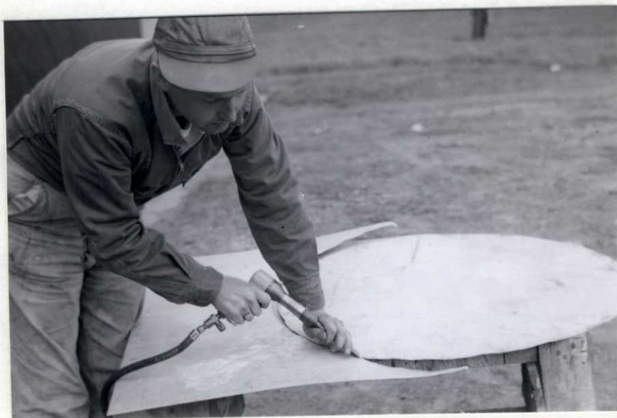
A riveting gun adapted as a tool to cut sheet metal and remove barrel ends by Clerk Dewey. This sheet metal was too heavy to cut with accuracy with tin shears but was readily cut with this tool.
