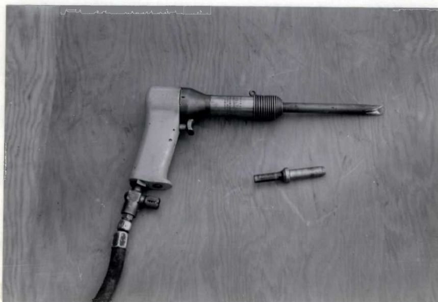
The gun fitted with a blank tool that can be purchased and altered to suit ones needs. The end of this blank was shaped on a grinder as shown. A normal riveting attachment is shown below. (Surplus property.)
