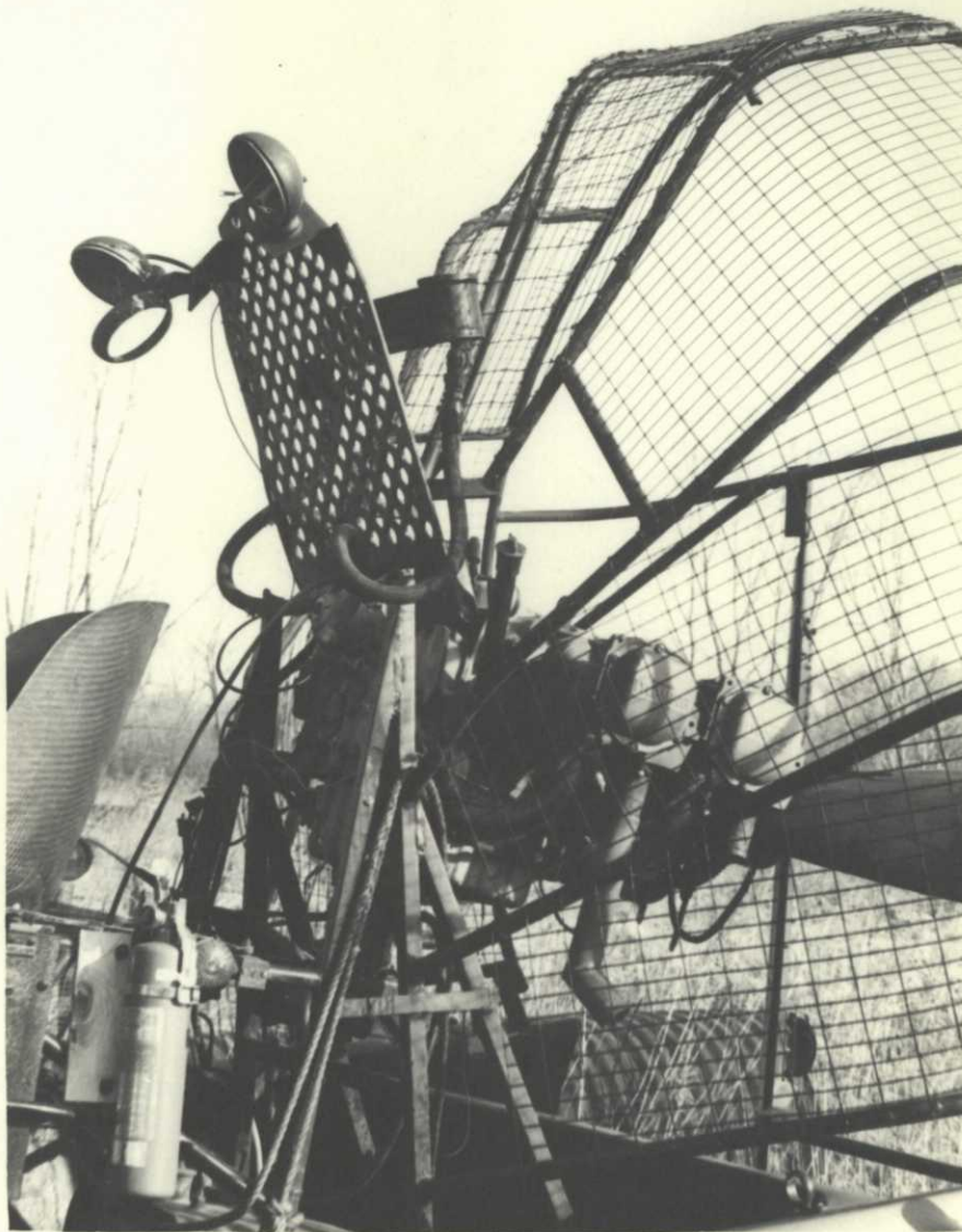
The 1965 "Aircat" airboat had the audacity to fail us on the Canadian waterfowl banding assignment in New Brunswick! A rebuilt engine had been installed and the hull and trailer rebuilt but the engine mount and frame broke from metal fatigue. Note the angle of engine, guard, broken lights, etc.
