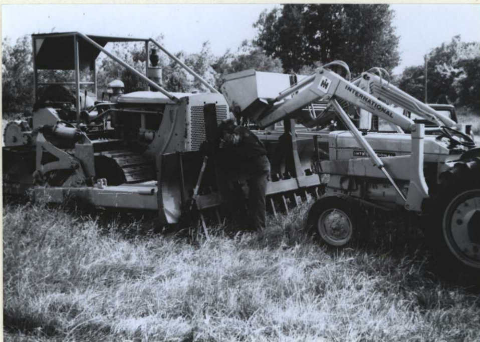
Attachment brackets being welded on the blade of the Caterpillar D-7 to support an H & L Brush Grubber attachment. This attachment is readily put on and off-attaching by two pins through the vertical arms. Various holes in the vertical arms permit its use on a variety of sizes of bulldozer blades.
