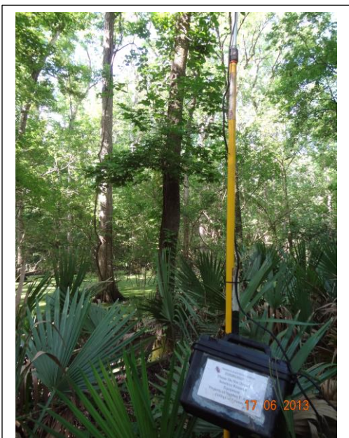
Figure 3. Grab and go kit with painter pole and cables showing, deployed in a control unit at Tensas River NWR.
