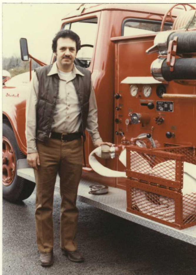
Fire Chief DeJulio showing new Siamese connection for use with fire hydrants. 10/82-10 DJS
