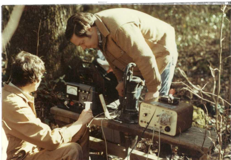
U.S.G.S. "Oxygen expert", Wayne Webb and FWS Biologist Garrett measure dissolved oxygen in a observation well on the transition zone study.
