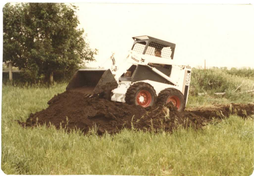
Figure 8. Hyink buries old fence on Madison WPA. The Bobcat is a handy piece of equipment for the clean-up of rock and junk piles existing on WPAs throughout our district.
