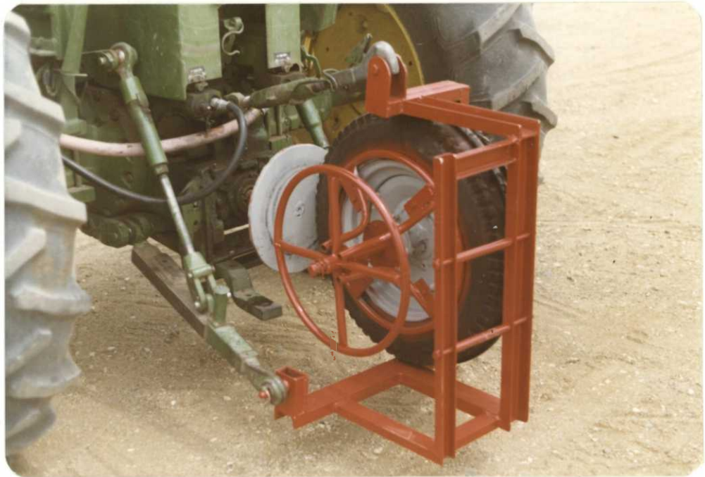
#22 - Barbed wire roller custom built by maintenance helper Jim Steinmetz. Old wire is guided through center square onto spool which is driven by rubber tire on PTO. The square guide makes it impossible for the wire to slip off of the spool while winding. 81-22 FGM
