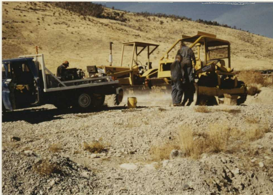
Class members from NNCC, Elko remove and replace cracked cylinder sleeves in the TD-14 dozer. FWC 10/80
