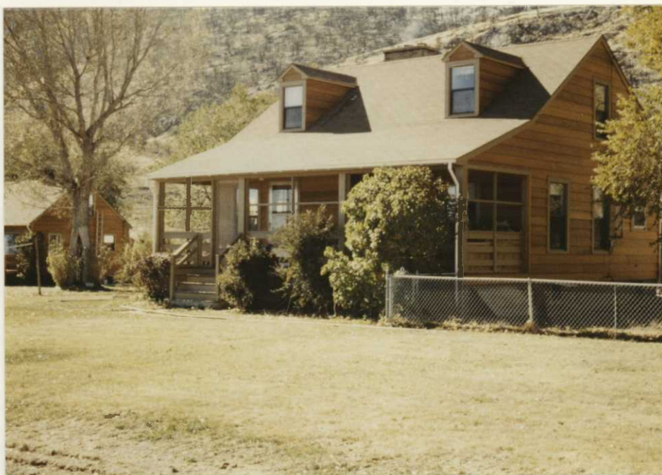
Quarters #8 and other refuge buildings were remodelled with red cedar siding and new roofs in earthtone colors. Several windows were also replaced with thermopane type. Interior was repainted by Johnson and Cameron in off work hours. FWC 9/80
