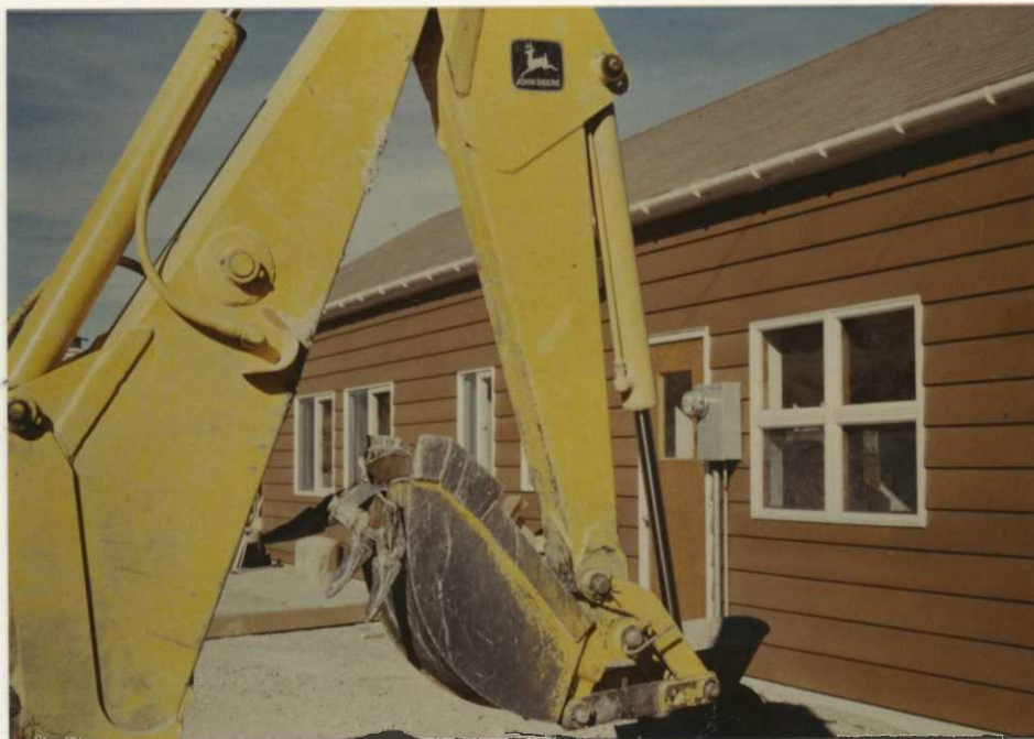
The condition of the backhoe bucket attests to the solidity of the "soil" in an August trenching operation. FWC 8/80
