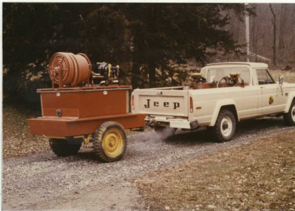
New fire pump (Pacific) mounted on old military trailer. 11/82 BH
