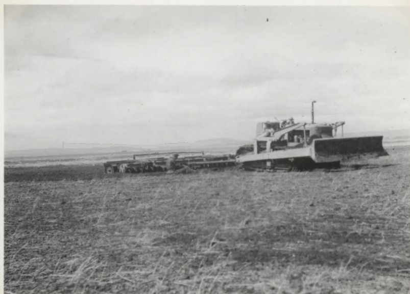
10. TD-11 tractor with two 12' offset disks in squadron - Fairchild Island. (Ramelli)
