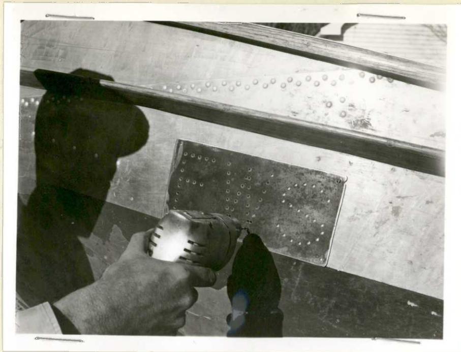
Identification of Service owned metal boats. (See Mid-year Progress Report, Management Improvement Program, Region 1, January 1955. III, projects completed. Page 7, Item 10. Metal Boat Marking Kit.) Drilling holes with 1/4" electric drill and template.
