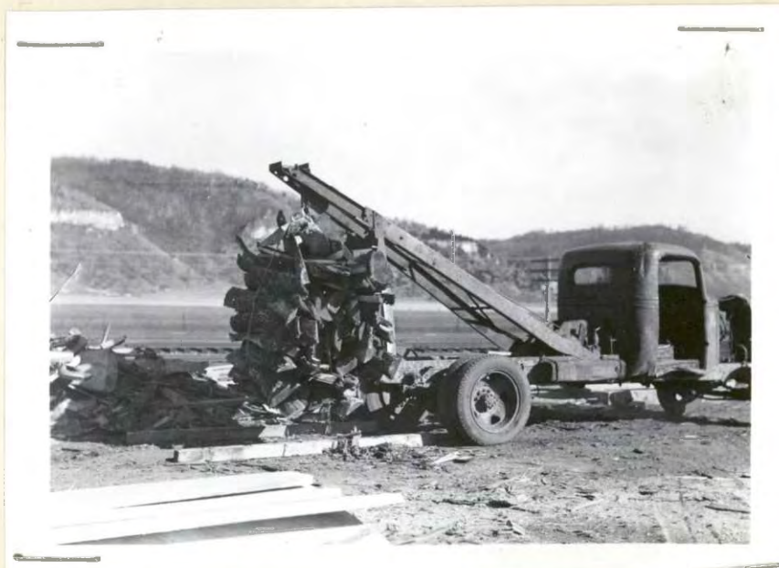
Truck converted for use at mill, handling slabs. This type vehicle is also used to handle logs, cross-ties and other material. It can be used in the woods to assist in the logging operation. Hutchison Bros. mill. March 1946.
