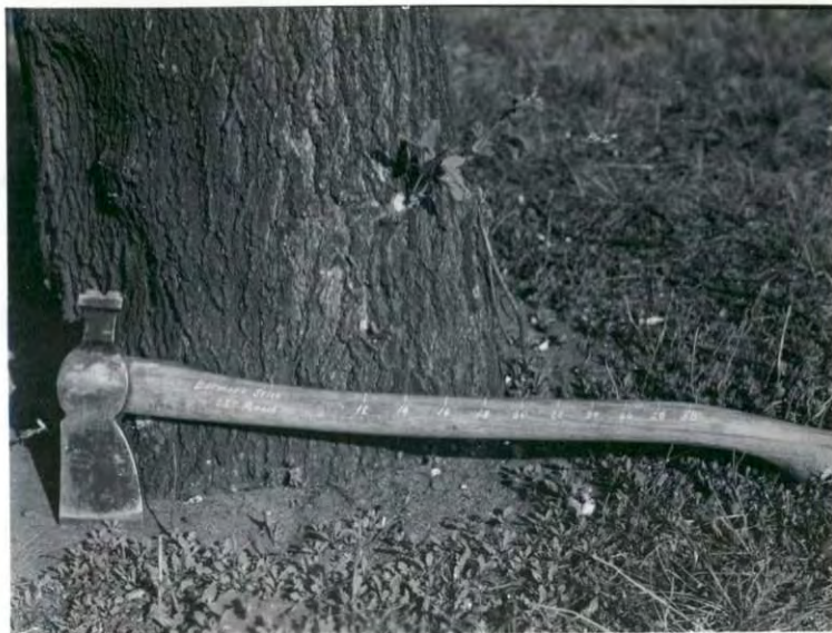
Biltmore stick markings on marking axe to facilitate measuring tree diameters when marking trees for cutting.
