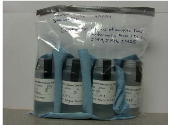
Figure 6. Absorbent material placed between the primary sample containers and the secondary bag.
