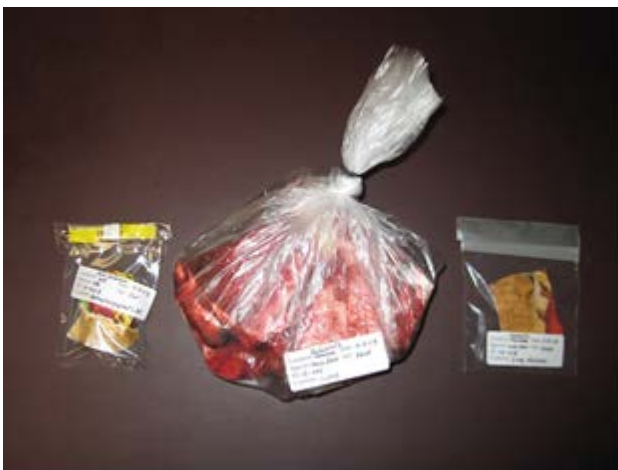
Figure 3. Examples of properly sealed and labeled primary sample bags using tape, twists, knots and zip ties.
