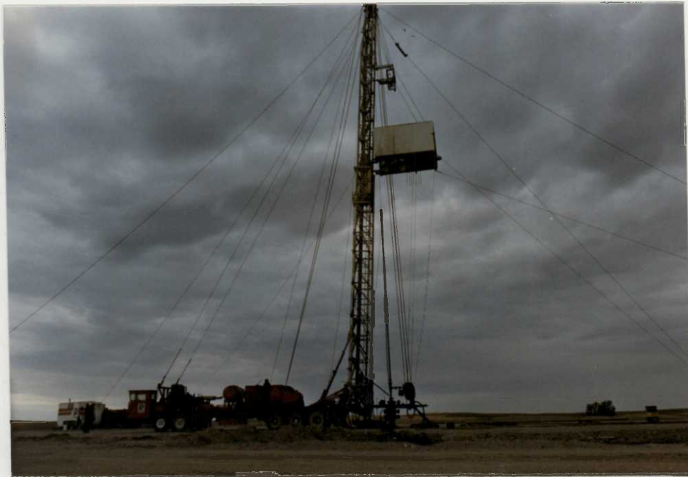
Figure 26. Next step in process is a "workover rig" in NE 14-153-84 on W207x. (11/88. RA. 10-88-23)
