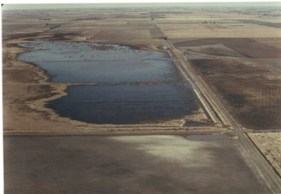
Fig. 11. An aerial view of the restored wetland due to BLHP dike work which keeps water on the WPA from "going down the drain" - that is a legal tile installed in the early 1900's. W.W.
