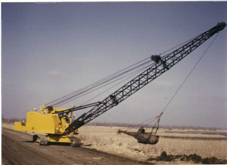
Lorraine 3/4 yard dragline obtained excess from the Air Force last year with less than 200 hours on it. The new center section of boom was purchased this year to extend the boom length to 45 feet. BH 11/86
