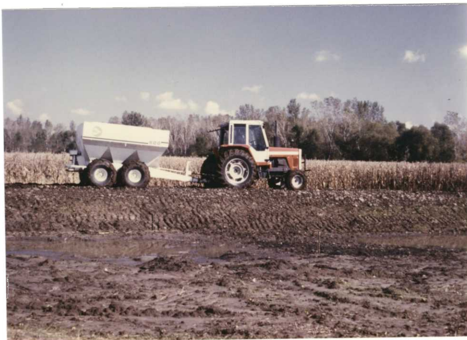
Seeding wheat to stabilize new moist soil unit levees. BH 10/86
