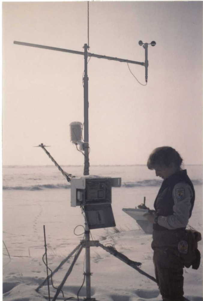
Utah State University installed a weather station that continuously records coded data to a tape recorder.
