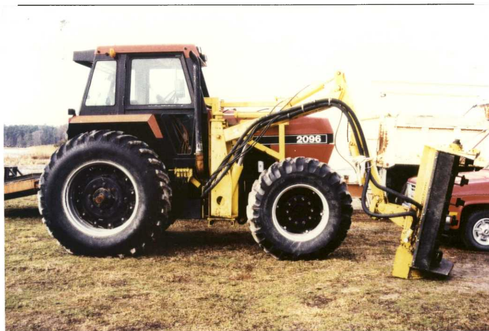
Fig. 134. Case 2096 tractor with flail mower for dike slope mowing. This type of mower was totally inadequate for mowing dikes at Blackwater. (GCH)
