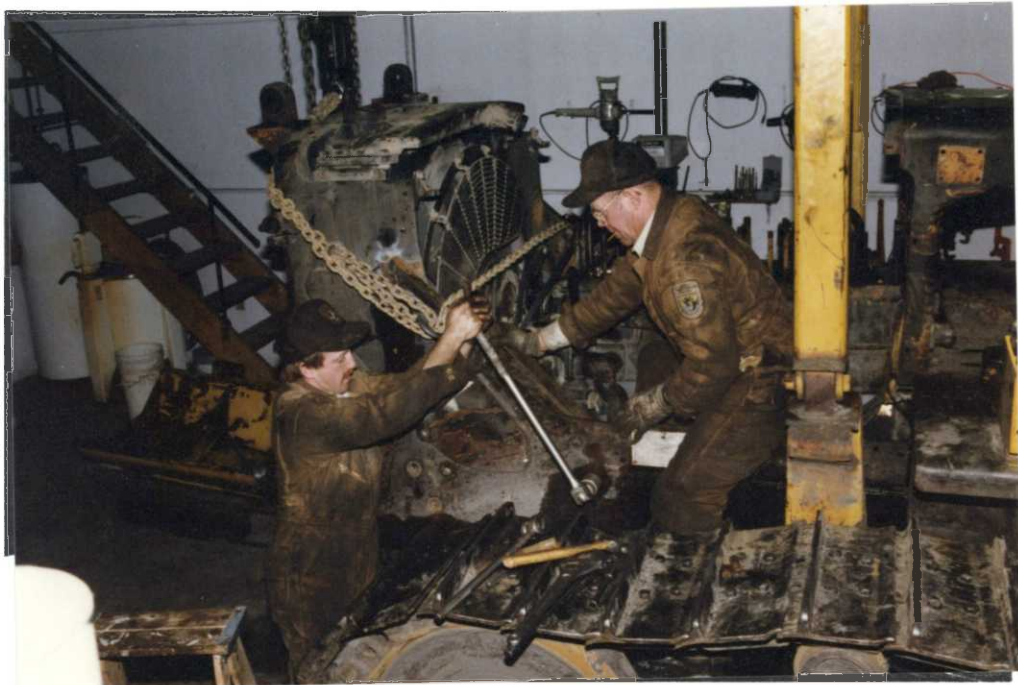
GERALD FELCH AND DAVID GINS OVERHAUL D-7 CAT OBTAINED ON SURPLUS FROM BROWNS PARK NWR.
