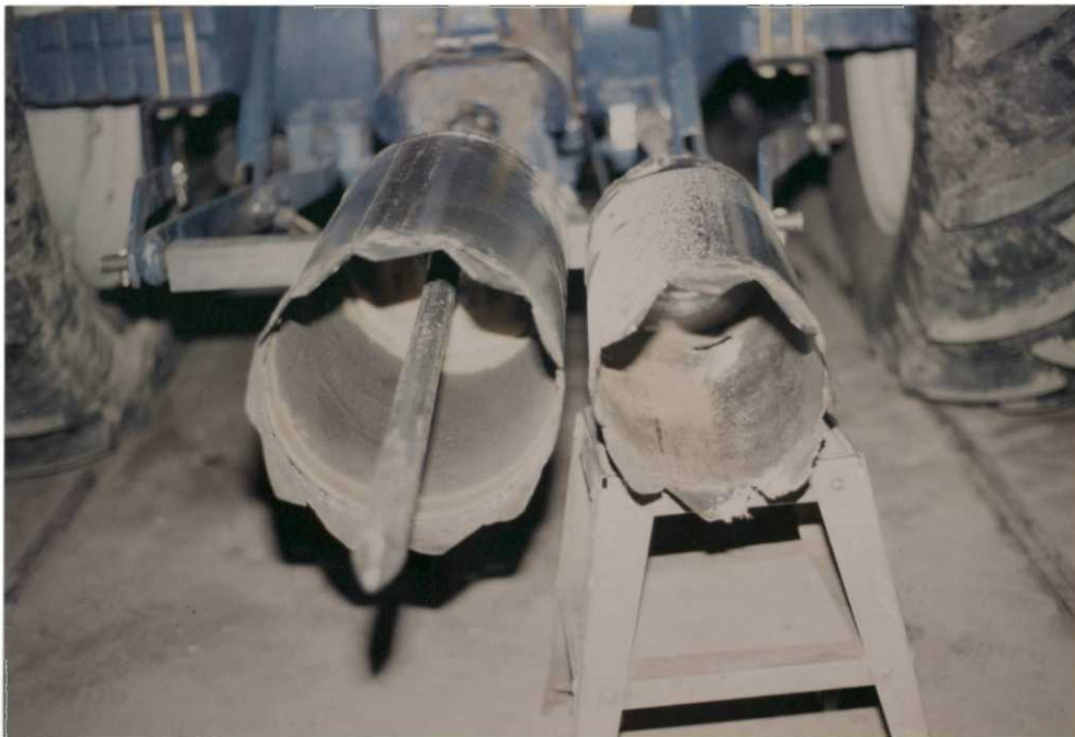
DUCK NESTING SUCCESS IN CAVITIES OF ROUND BALES LED TO THE DEVELOPMENT OF A LARGER DIAMETER BALE DRILLER. THE NEW ONE IS ATTACHED TO THE TRACTOR WHILE THE OLD ONE IS NEXT TO IT.
