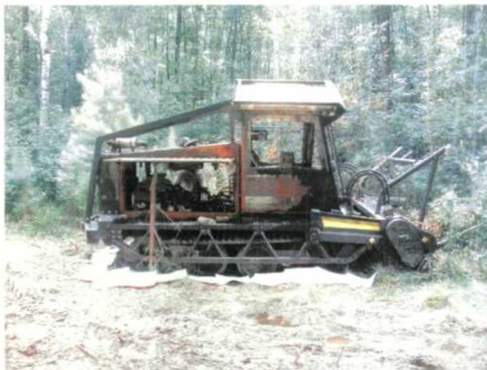
The Refuge's Gyro Trac caught fire due to an apparent electrical shortage and was destroyed. TC
