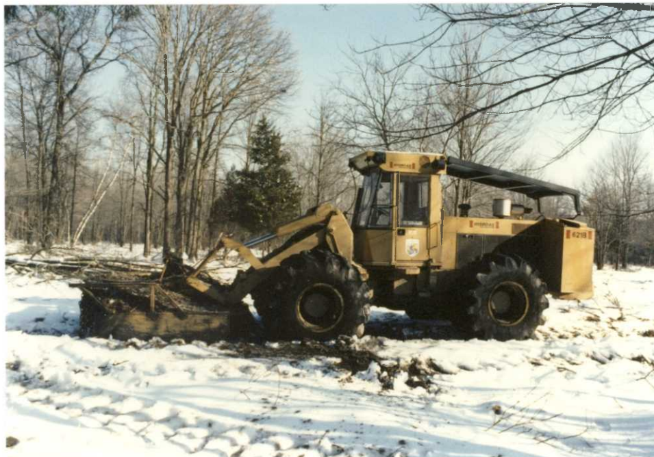
Hydro-ax with rotary cutter attachment (TM)
