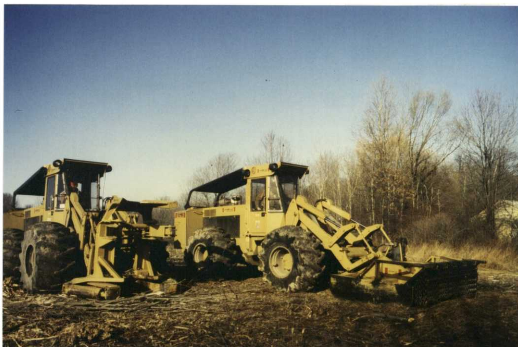
The Great Swamp and Iroquois's hydro-axes worked in tandem. Feller-buncher (L) Rotary cutter (R). (TV)
