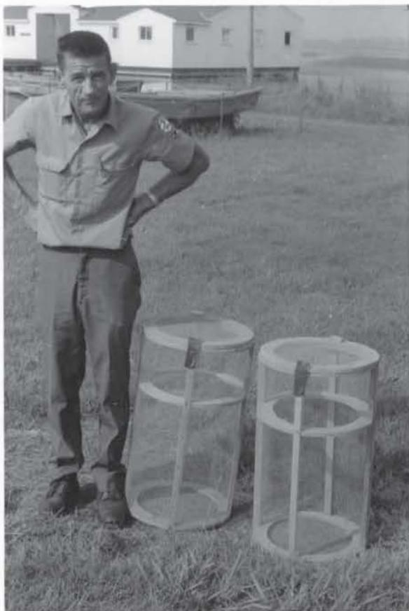
Type of cylinders used at Back Bay NWR (left) and Chincoteague NWR (below) into which transplanted loggerhead turtle eggs were placed and buried.
