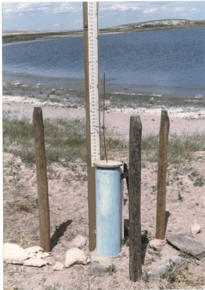
Figure 6. Float gages were installed on Gaffney and Homestead Lakes. The gages allow us to record water elevations well below existing staff gages. exp 21, 7/19/91. MJR
