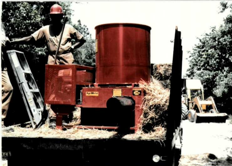
This straw grinder/blower cut the time required to mulch erosion control projects considerably. (88NR-44, 6-88, Cartlidge)
