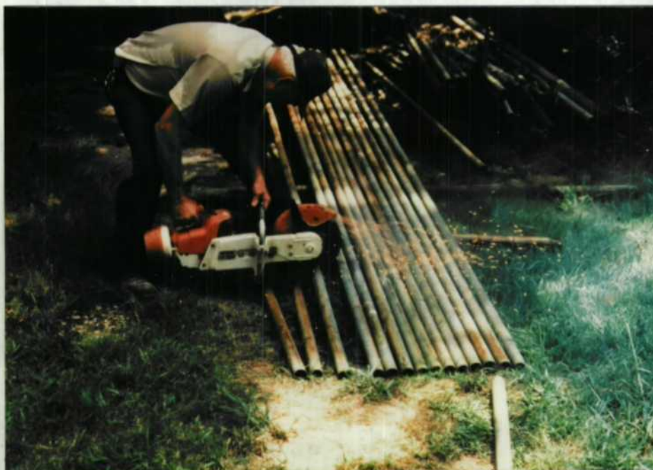
Volunteer Clyde Mitchell cutting some of more than 500 sections of 2" diameter galvanized pipe used to more permanently mark over 80 of the GTR study plots.
