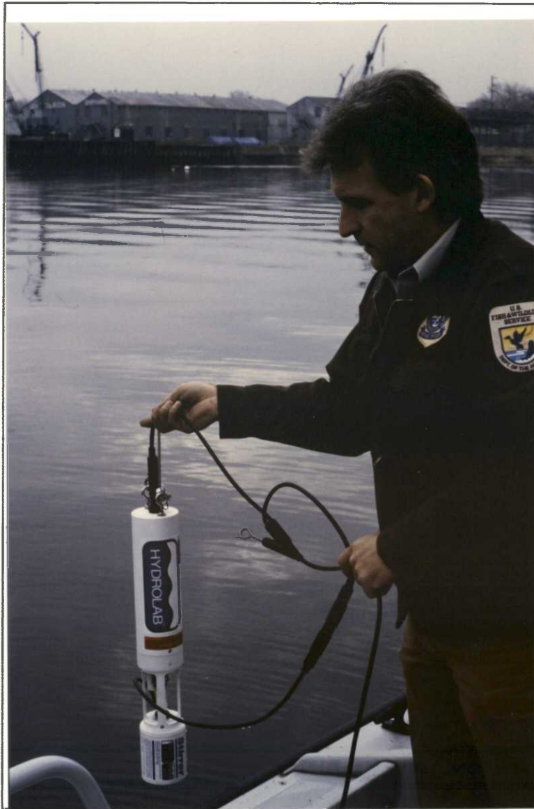
EEO Marto using Hydrolab probe to measure various water parameters at the Refuge. RWP-1993
