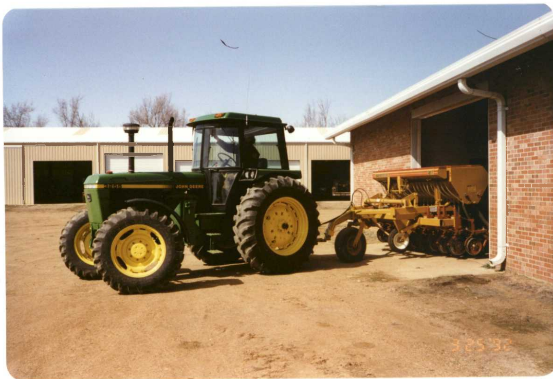
Figure 10. New 3255 JD tractor ready to go seeding native grasses with the Haybuster drill (92-300,exp3,ES)
