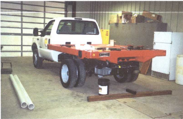
Figure 52. Two new fire trucks were also added to the vehicle fleet in 2001. This truck is being prepared by the Refuge Crew for the fire tank/pump to be installed on contract. 01-GM
