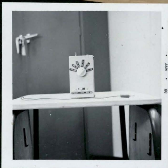
Volt-ohm-meter is used to adjust power output on transmitting collar.
