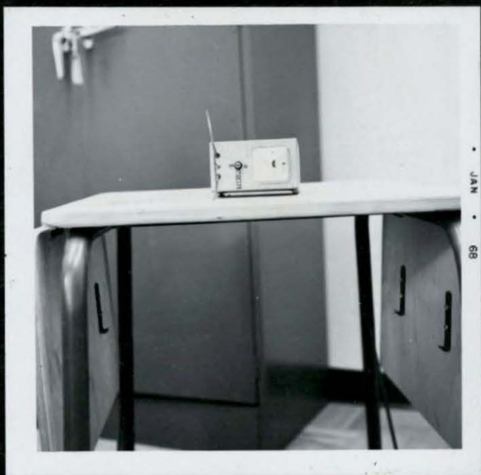
Volt-ohm-meter is used to adjust power output on transmitting collar.
