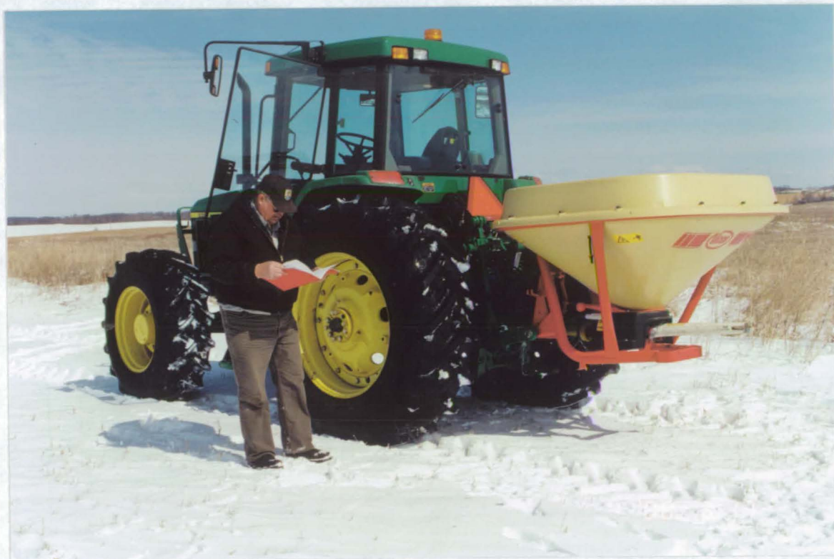
#00-02-11. Tractor Operator Bob Scherzer adjusting new Vicon snow seeder. Snow seeding requires no seed cleaning, allows use of simpler machines, and cuts personnel time. (MTM 3/00)
