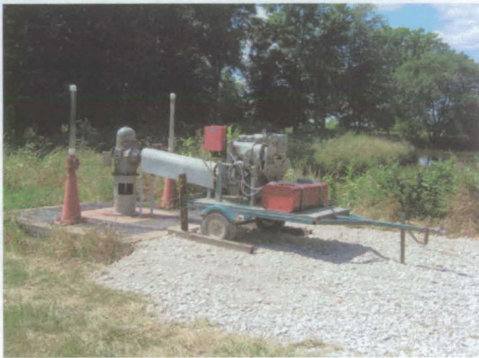
Portable Moist Soil Unit pump used for M.S.U.'s 3 and 4. Photo by David Peters.
