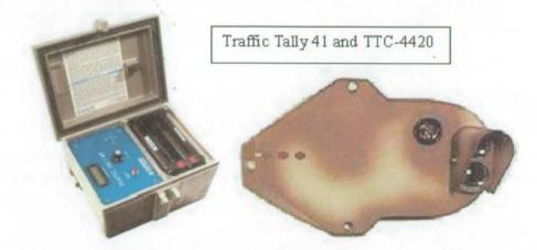
Inductive loop counters count vehicles by a buried inductive loop (wire) under a road bed. The loop gives off a slight magnetic signal and when a large metal vehicle passes over that loop the counter counts. The system has proven successful and will operate for over a year on a set of batteries.
