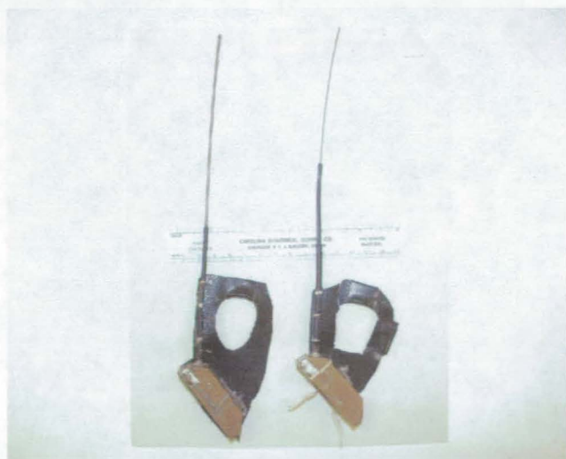
Satellite collars weigh 20 grams, 5 more than the conventional radio transmitter pack, consequently only adult males have sufficient body weight to carry them. GH
