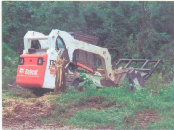
Randy operates the new Bobcat with a forestry tool attachment to grind up locust stumps, August 2008.
