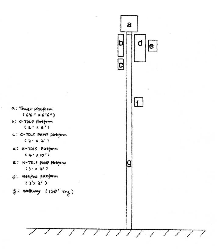
Platform Construction and Walkway cross section
