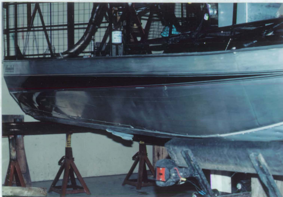
The airboat borrowed from Sherburne NWR with a tear in the plastic covering the bottom of the hull. The area of the tear was cut out and a new piece of plastic rivited onto the hull. 92-45 8/24/92 BLA
