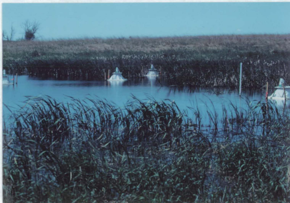
Emergence traps funnel aquatic invertebrates into collection jars for research into the effects of insecticide spraying. 92-9 6/4/92 BLA
