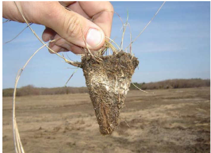
Figure 8. Marker horizon sample plug/core shows that after substantial burial, the marker horizon technique begins to incorporate both surface and subsurface processes (note root material above marker layer).
