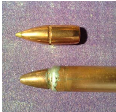
Figure 5.20. The bullet (top) and inserted in the copper tube (bottom).
