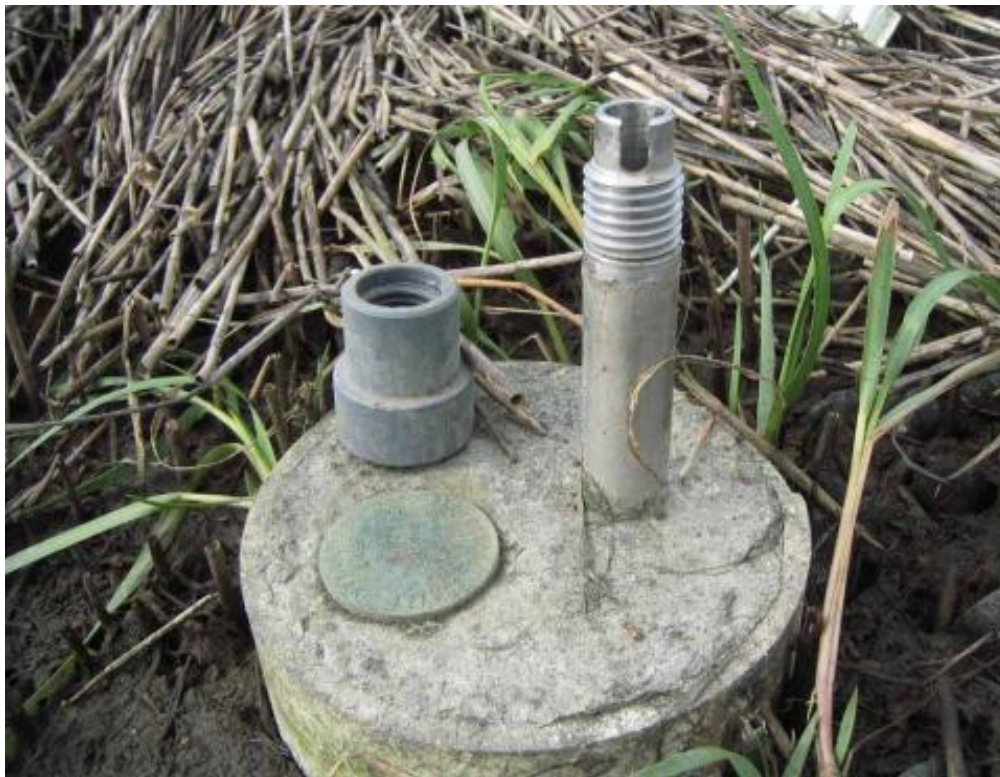
Figure 24. Deep RSET mark. The RSET instrument attaches to this mark via the threaded receiver. The grey cap is for protecting the mark when the instrument is not attached. The brass disc is for site identification and is NOT used for surveying.
