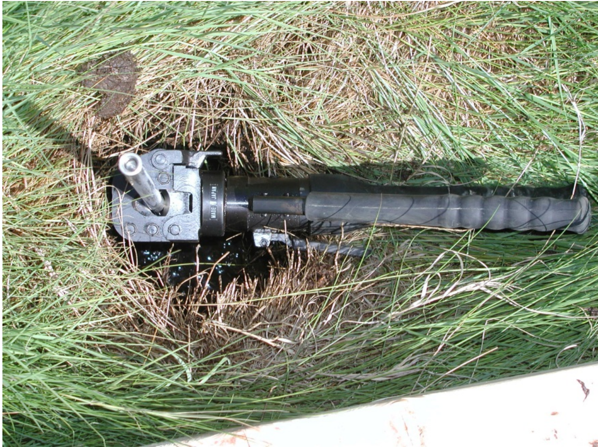
Figure 3.17. Hydraulic bolt cutter attached to the deep rod.
