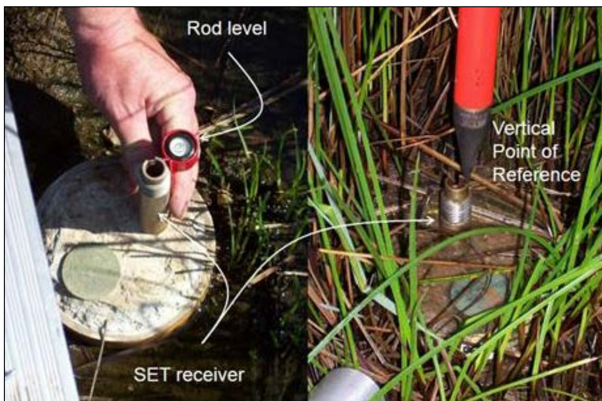
Figure 6.4. Finding the vertical point of reference (VPR) on a deep rod SET monument (left panel); central tip of GPS tripod on VPR. Note that the VPR is NOT the brass disk set in concrete next to the receiver.
