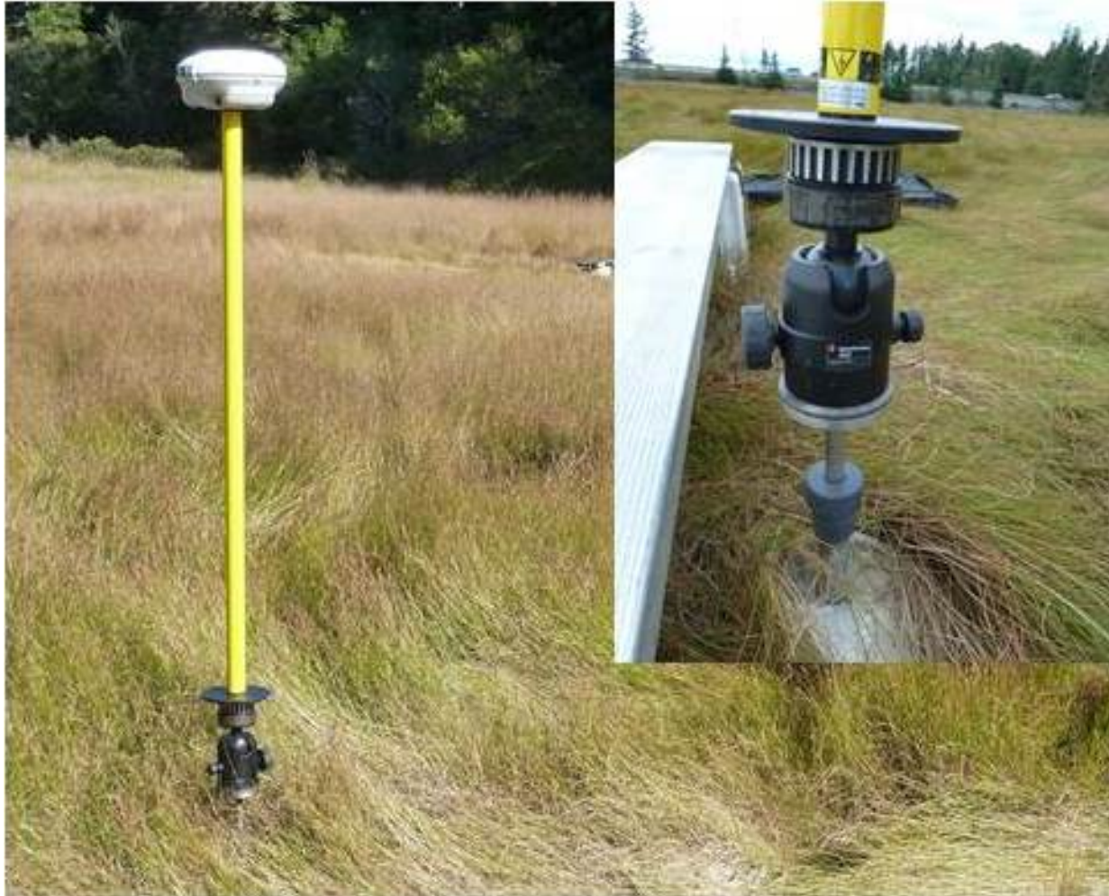
Figure 6.12. Custom adapter used to place GPS antenna atop deep rod SET mark.
