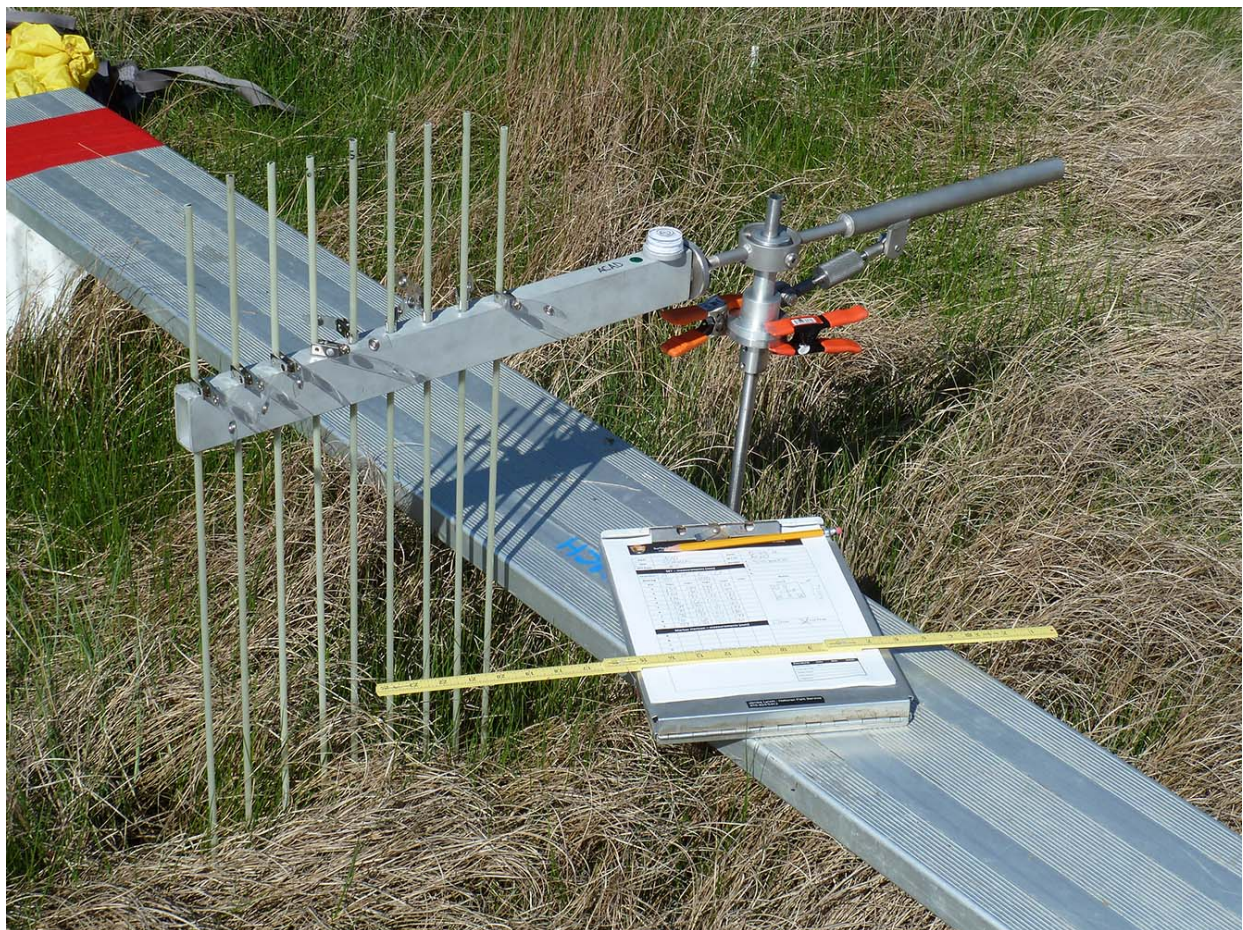
Figure 4.1. Rod SET attached to a deep rod mark (Acadia National Park, Maine, USA).
