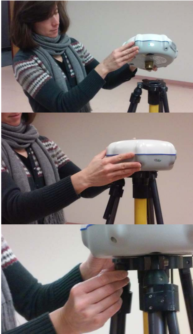
Figure 6.8. Placing GPS antenna on top of fixed height tripod.
