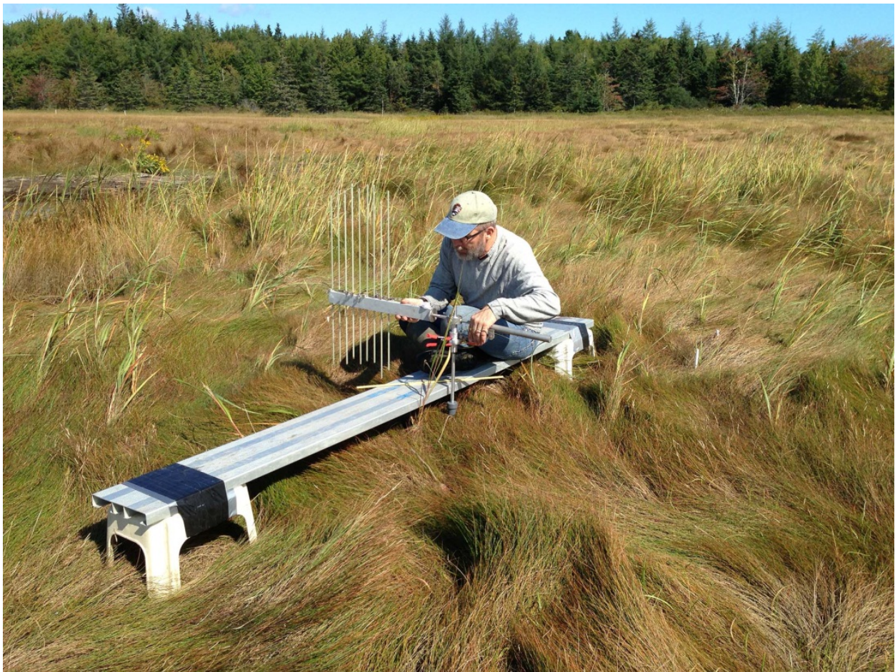
Figure 2.20. Temporary platform (Acadia National Park, ME, USA). Note the step stools are attached to the plank with duct tape.
