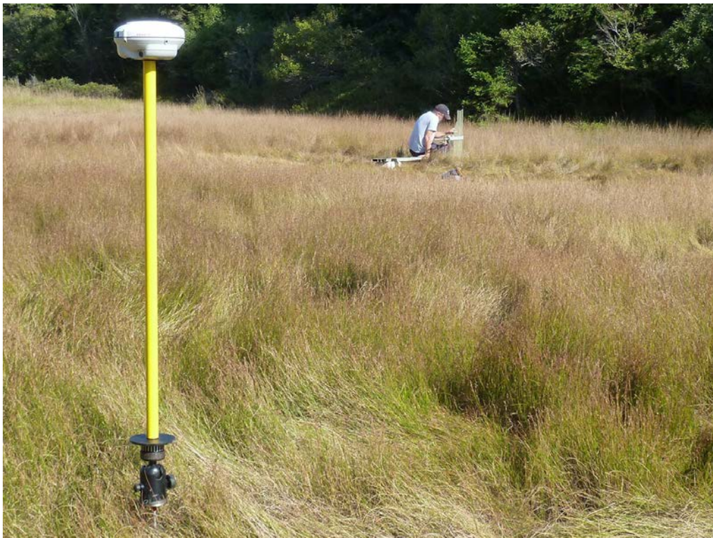
Figure 25. GPS receiver deployed on an SET mark for a static occupation (Acadia National Park, ME, USA).
