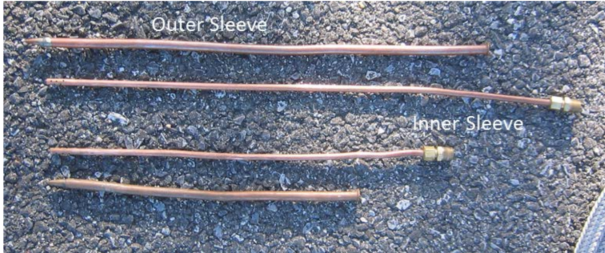
Figure 5.18. The “Bullet”: The inner sleeve and the outer sleeve.
