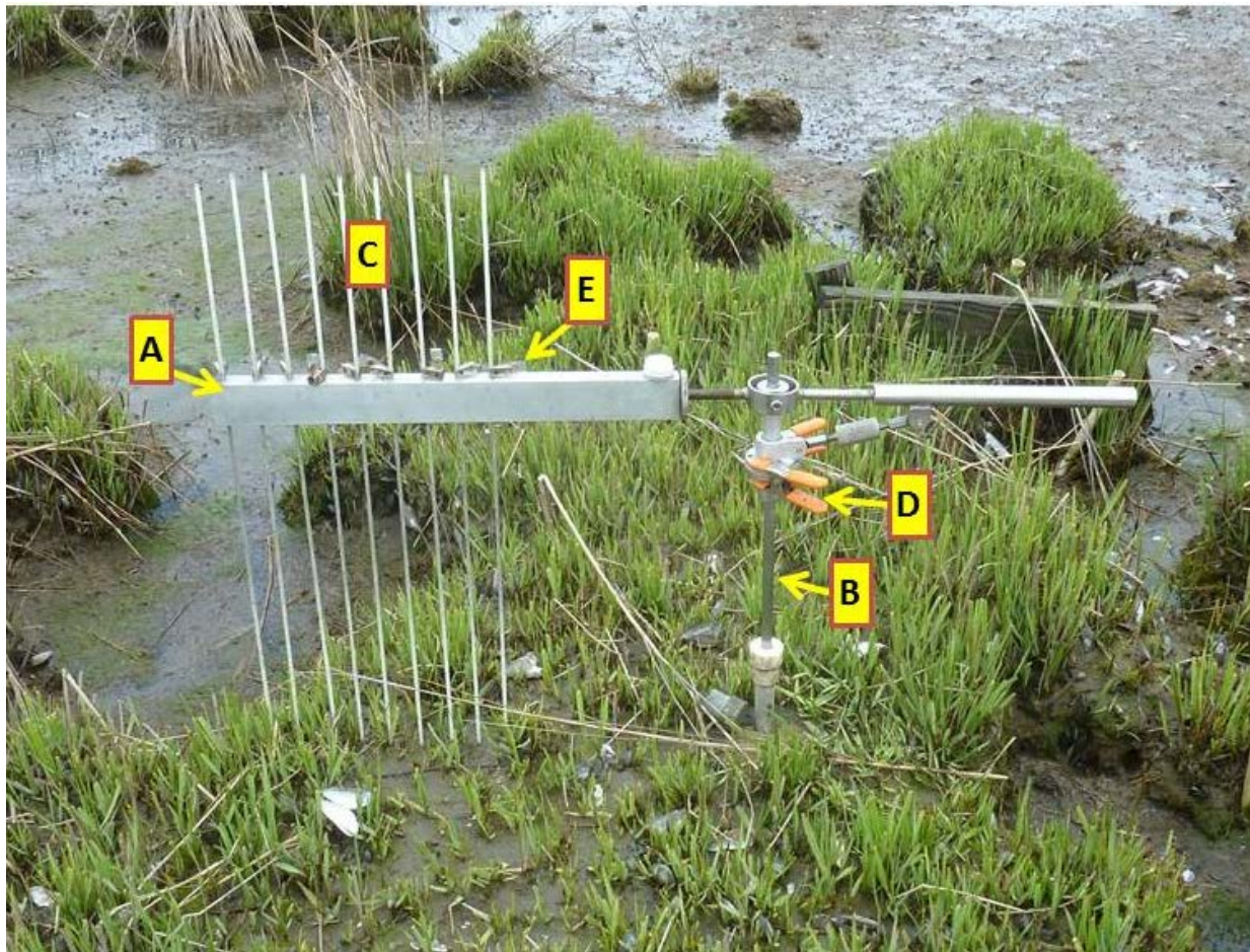
Figure 4.3. RSET instrument: A = Horizontal arm, B= Insert collar, C = fiberglass pins, D= Pony clamps, E = Badge clips.
