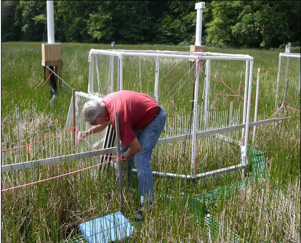
Figure 15. The Smithsonian Institution's "Monster SET" in operation. The RSET instrument, with a 4 meter long arm incorporating 100 pins, is able to cross both treatment (CO 2 enclosure = PVC structure) and control areas outside the treatment enclosure (Smithsonian Environmental Research Center, MD, USA).
