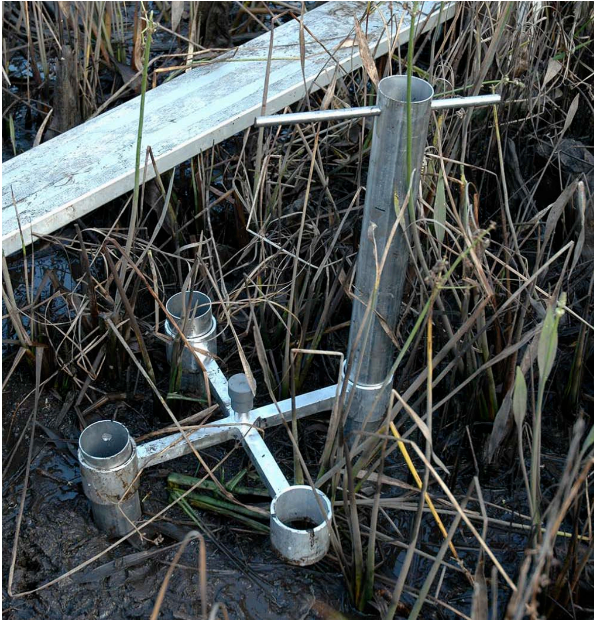
Figure 3.32. Shallow platform leg installation. Two legs have already been twisted into the soil. Note that the legs have a hole in the top to allow a section of stainless steel rod to be used as a handle to aid twisting the leg into the ground.
