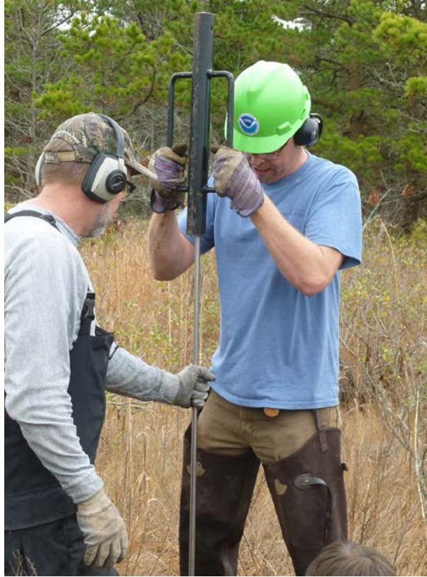
Figure 3.3. Hand pounder (Waquoit Bay NERR, Massachusetts, USA).
