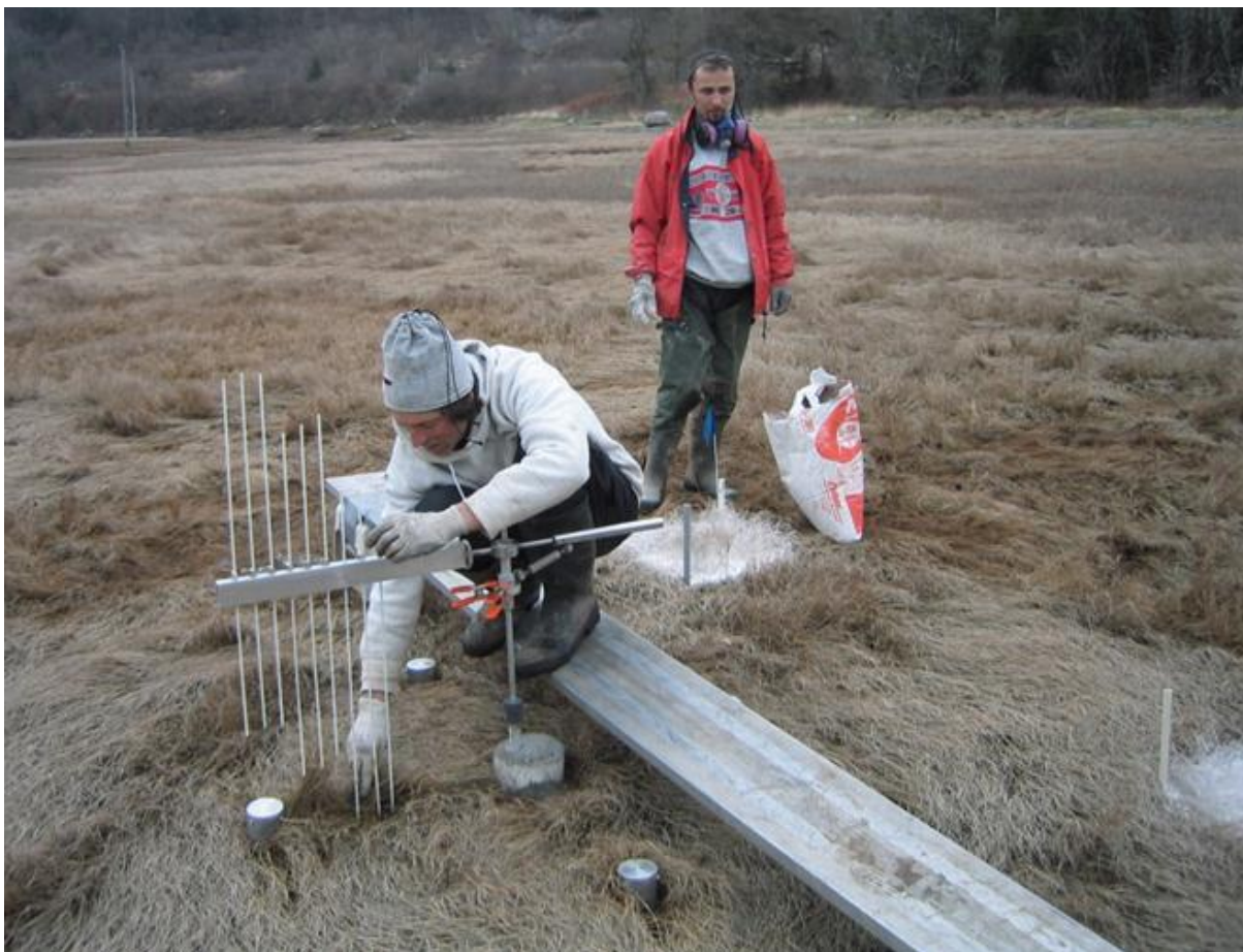
Figure 5.1. Establishing marker horizons at an SET sample station (Dipper Harbour, NB, Canada).
