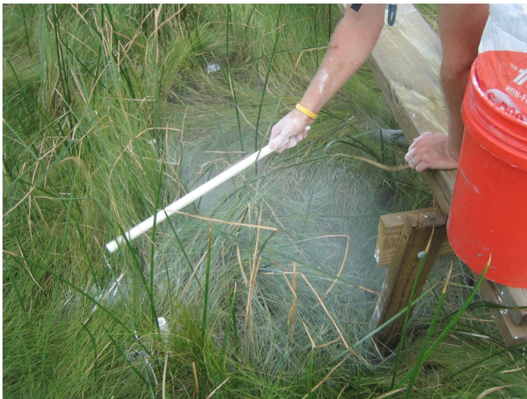
Figure 5.8. Knocking the feldspar off the vegetation (Bombay Hook, NWR, DE USA).
