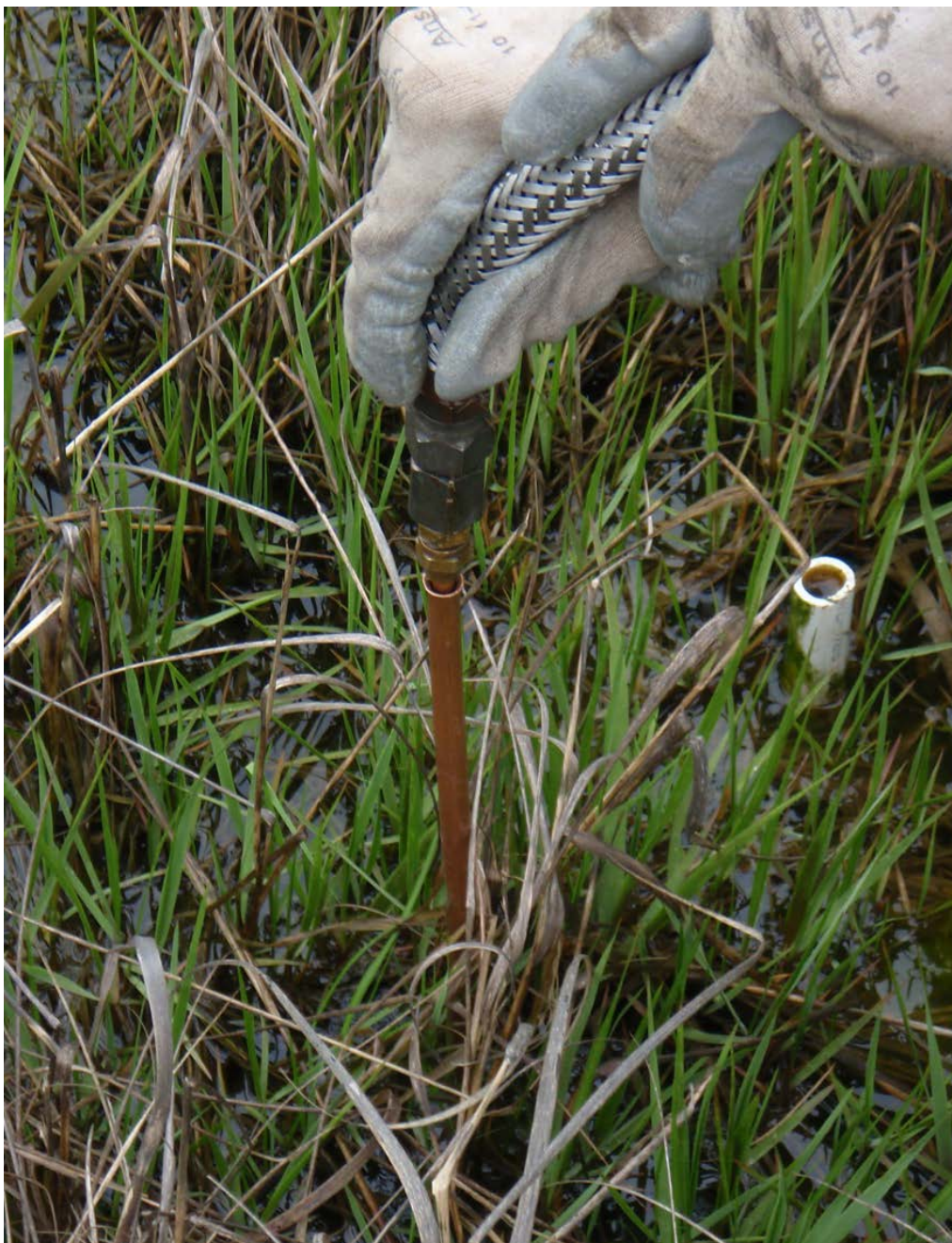
Figure 5.33. Bullet being inserted into the wetland sediment (before freezing).
