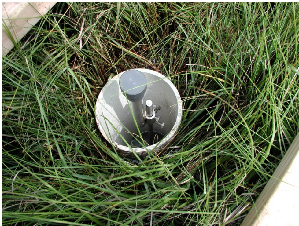
Figure 3.23. Receiver attached to the deep SET mark before cement is added.
