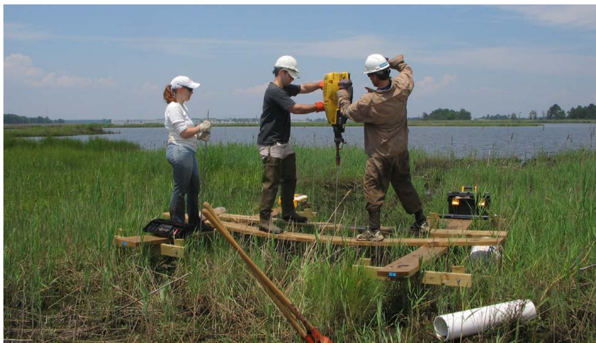
Figure 23. Installing a deep RSET mark in a Chesapeake Bay brackish marsh. In this example, a portable gasoline powered jackhammer is being used to drive rods. Note the permanent sampling platform installed to minimize human disturbance of the marsh surface where the readings will be taken. A removable, portable platform could also be used (Chesapeake Bay Environmental Center, MD, USA).
