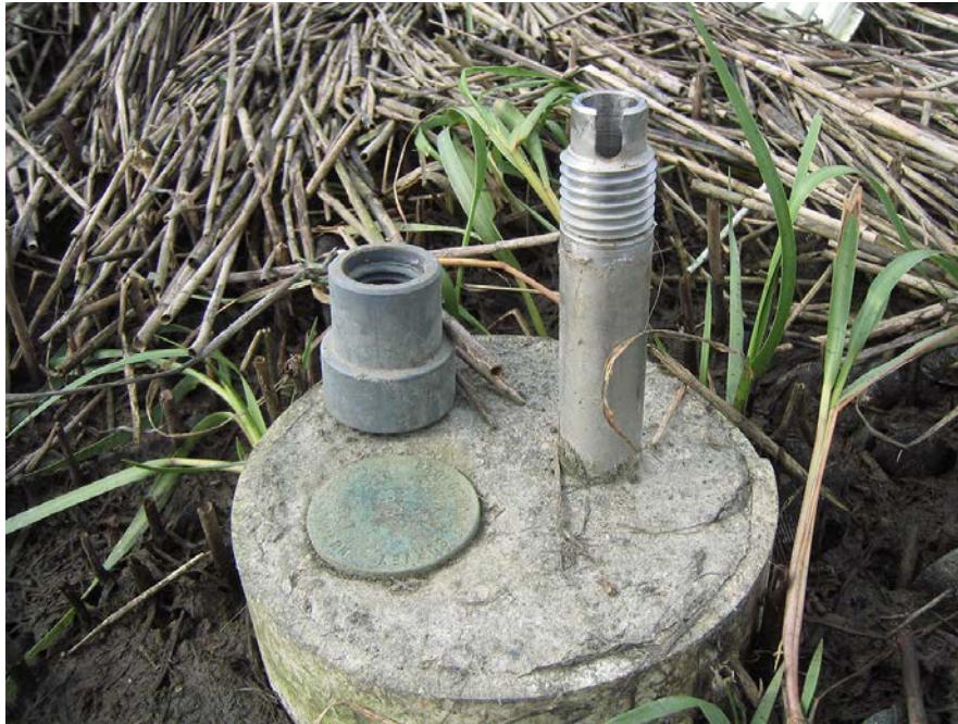
Figure 4.13. A receiver with cap removed showing the notch in the receiver; and the brass marker used to ID the SET mark
