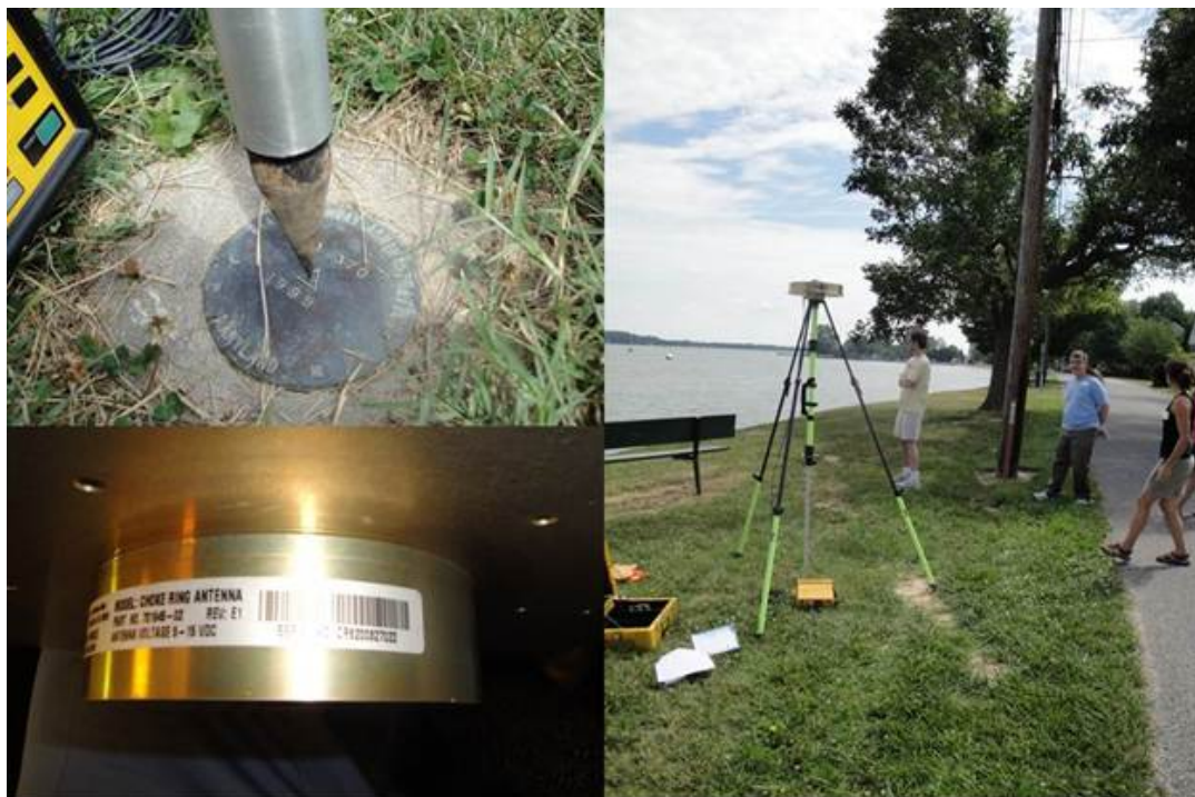
Figure 6.14. Photo-documentation required for a static GPS observation. Upper left: photo showing placement of GPS tripod over VPR of survey mark. Right panel: horizon photo showing deployment of entire GPS static assembly (GPS tripod, antenna, and receiver). Lower left: close-up of GPS antenna identification information.
