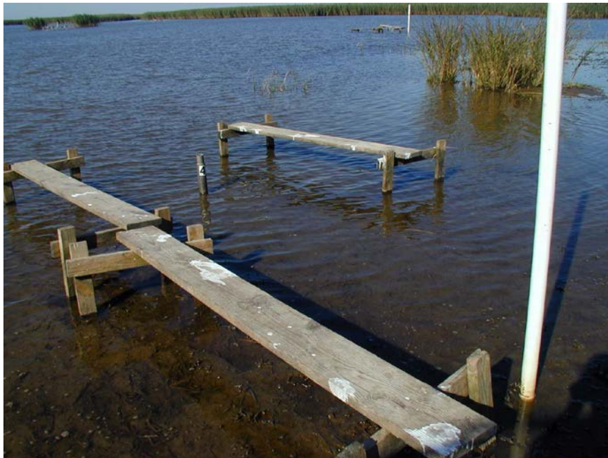
Figure 2.5. A permanent platform in a shallow pond (Delta NWR, Venice, LA, USA) with an original pipe SET mark. Note the mark is raised above the water to accommodate the SET, which requires longer SET pins to reach the water bottom.
