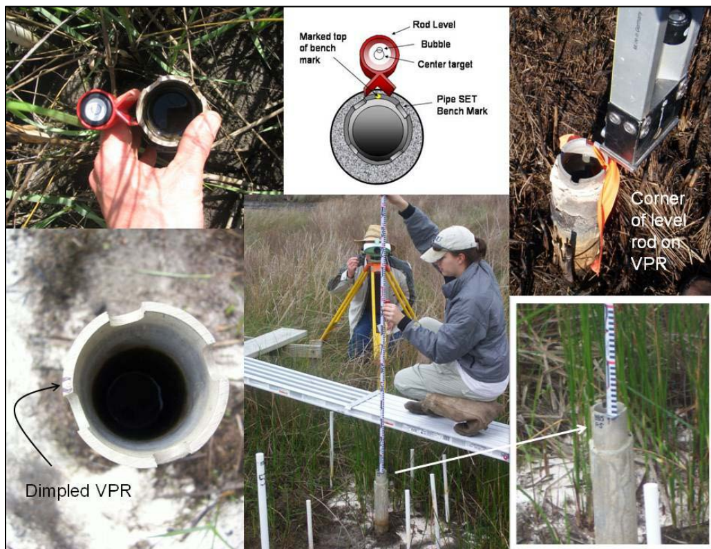
Figure 6.21. Example showing how to identify and level to the Vertical Point of Reference (VPR) of a pipe Surface Elevation Table (SET) mark.
