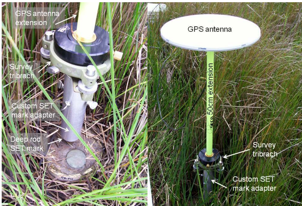
Figure 6.11. Custom adapter used to place a GPS antenna on a deep rod SET mark for a static GPS occupation.
