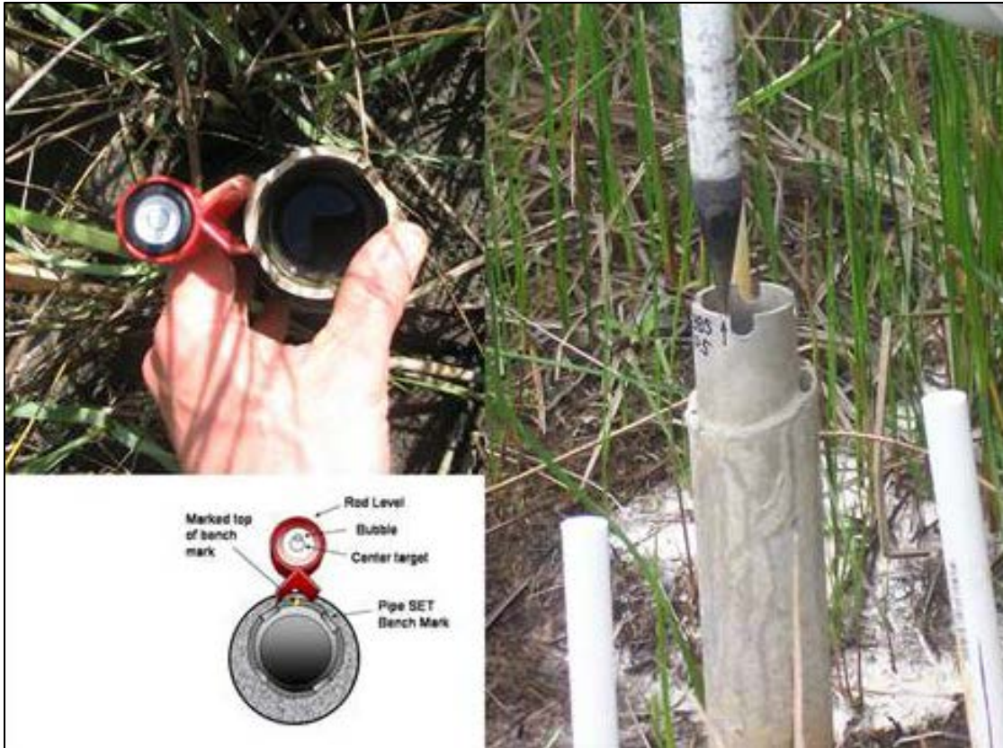
Figure 6.5. Finding the vertical point of reference (VPR) on an older, first generation SET pipe mark using a rod level (bubble gauge).
