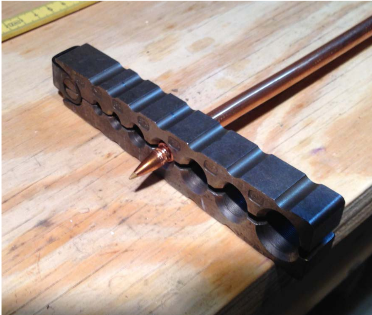
Figure 5.26. Compress the copper tube and bullet.
