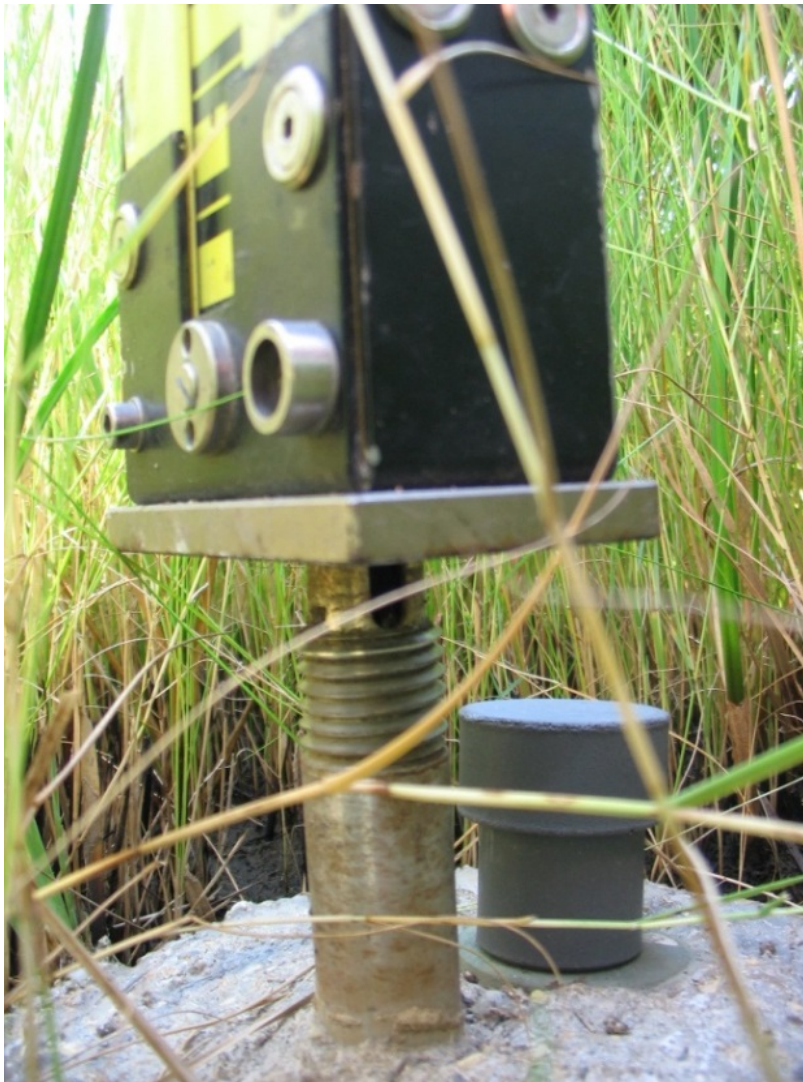
Figure 6.20. The base of a level rod is usually sufficiently large as to automatically find the top-most side of a typical Rod Surface Elevation Table (SET) monument.
