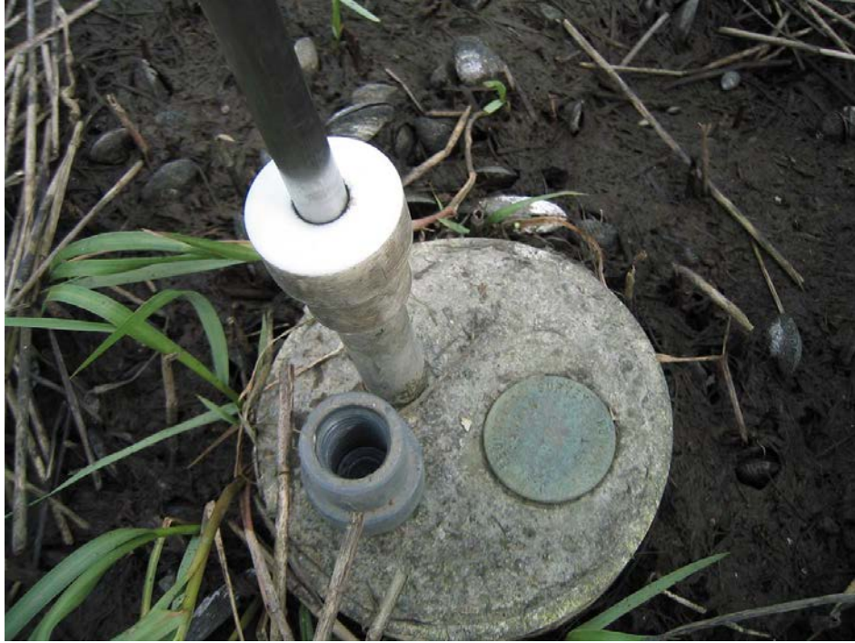
Figure 4.15. Receiver and RSET connected.
