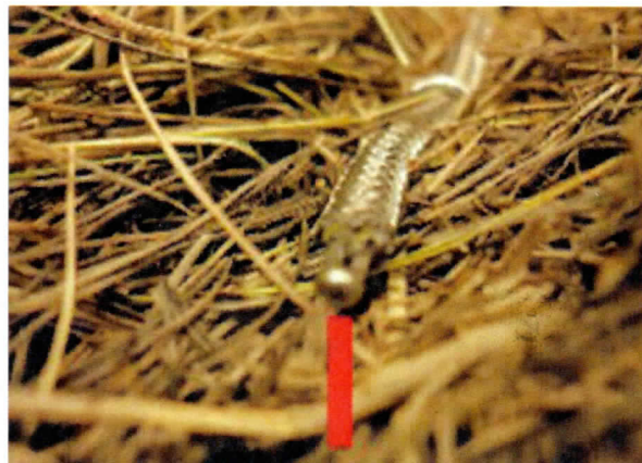
Thermocouple wire pinned down to the ground. Red line signifies 2 cm gap between ground and tip.
