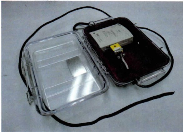
Fully Set-up Quick Deployment Thermocouple
