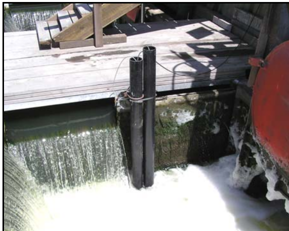
Figure 2-1: Datasonde holder within Weir Structure
