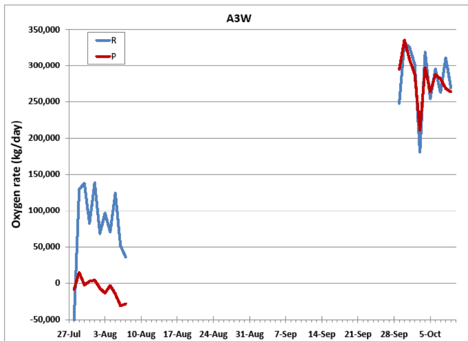
Figure 1. Comparison of the computed daily oxygen production/consumption rates of photosynthesis (P) and respiration (R) for pond A3W during both study periods. Respiration rates are presented as positive values to allow for easy visual comparison.
