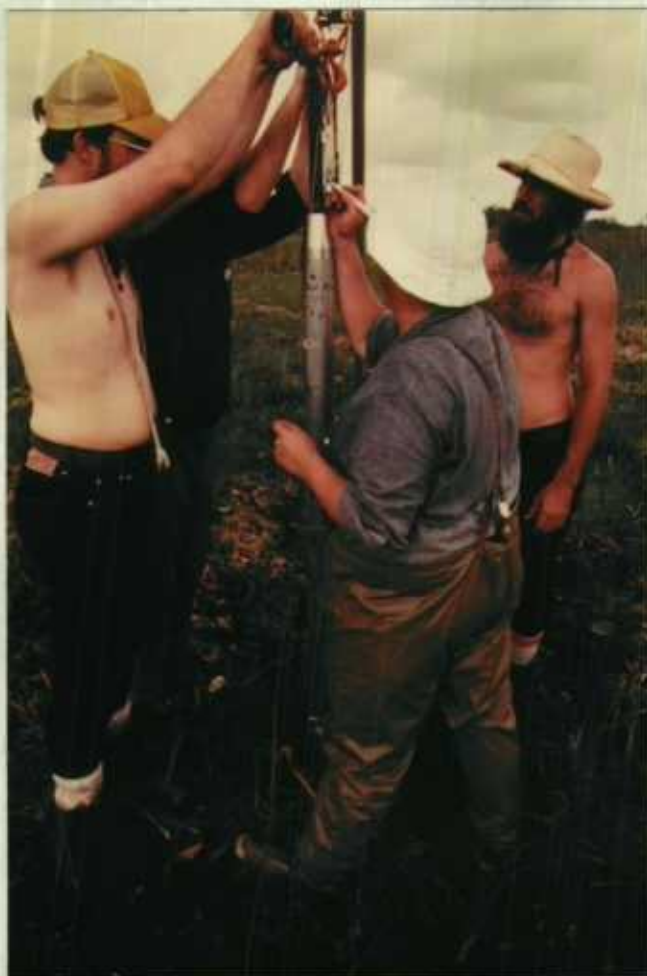
Researchers taking peat core samples for analysis. (Staff) 52-OKE-79
