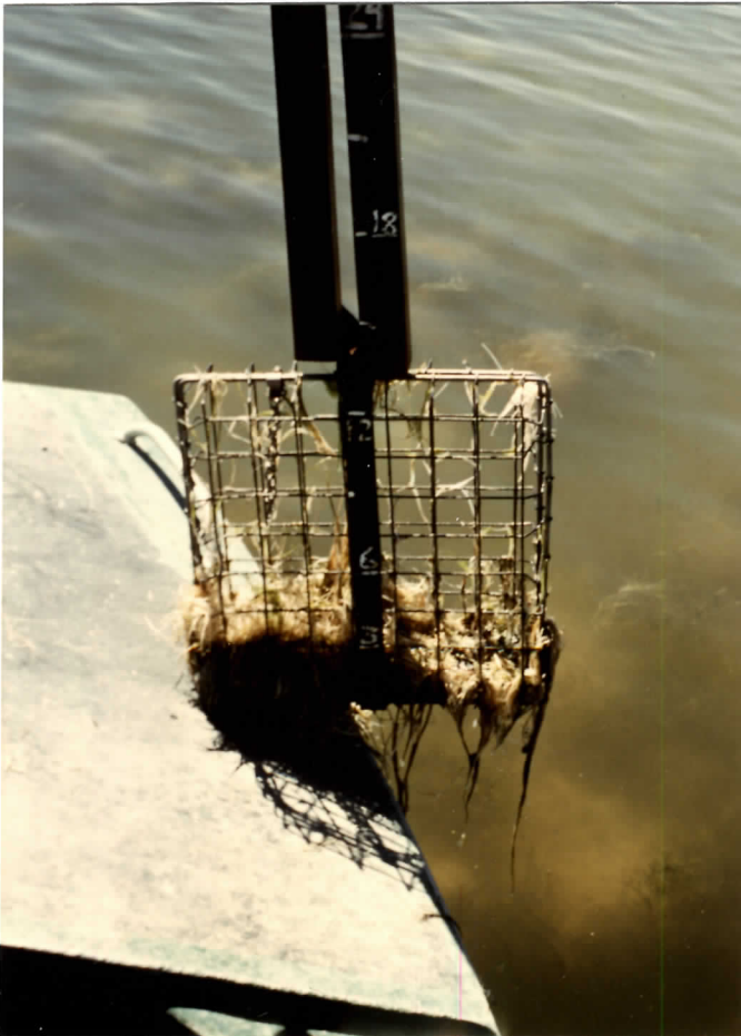
Figure 3. Sampling submerged vegetation using tongs
