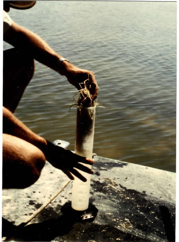
Figure 4. Measuring the volume of submerged vegetation by displacement in a graduated cylinder.
