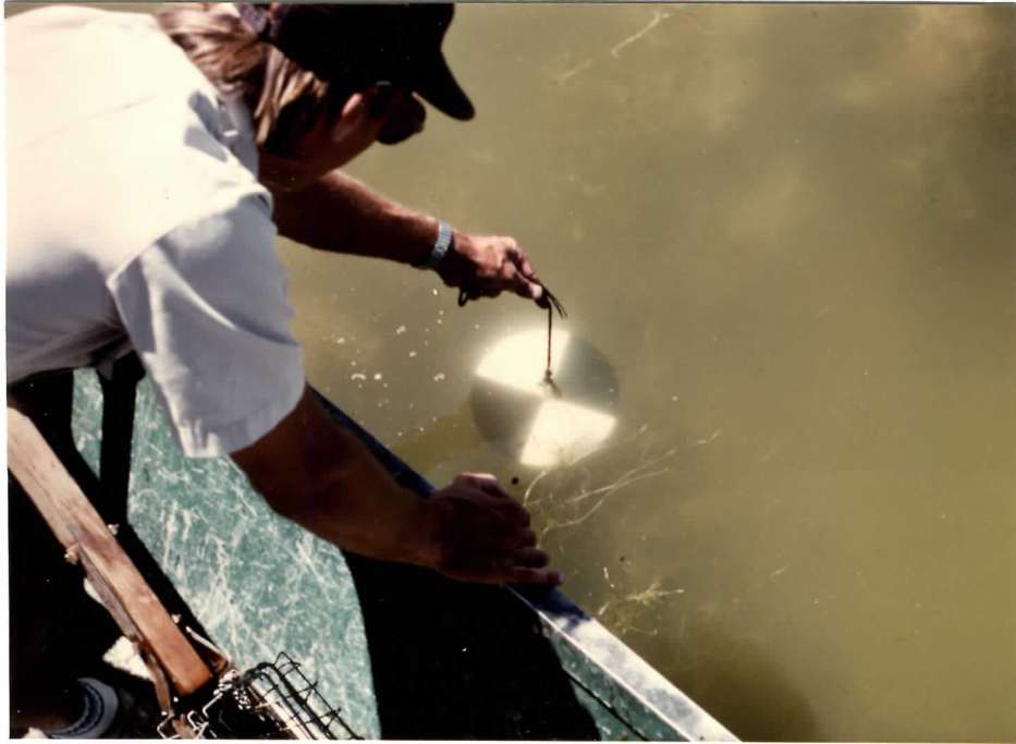
Figure 2. Using a Secchi disc to measure water turbidity.
